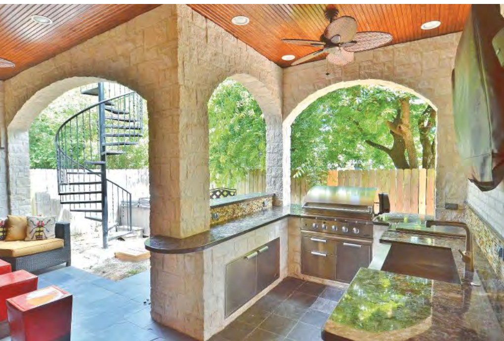
The bigger the area the higher cubic feet per minute (cpm) fan needed, Bawden explains. Two fans (above) are strategically placed in this under-deck area.
